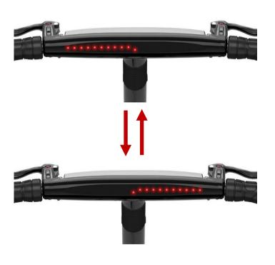
5.1. The Gocycle dash will alternatively flash all LEDs on the left and all LEDs on the right.
