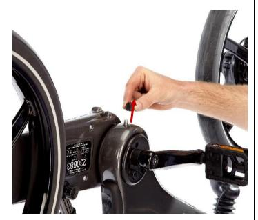
2.1. Remove the rubber cover and M8 nut
