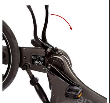
2.3. Attach the kickstand in the orientation shown. The legs close towards the **front** of the Gocycle.
