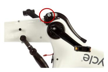
3.1 Locate the bolts on the Kickstand main body.
