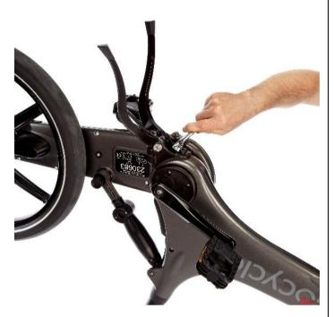
2.5. Use a 13mm spanner to tighten the nut to 20Nm.
