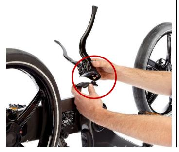
2.2. Open the Kickstand carefully. Align the kickstand rubber.
