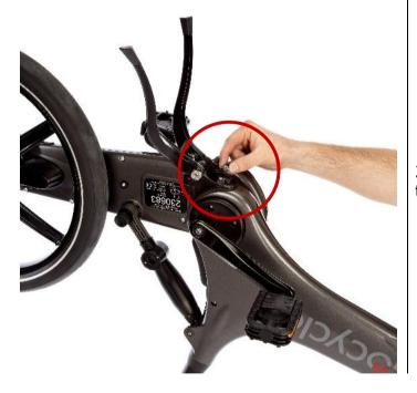
2.4. Thread the M8 nut onto the screw
