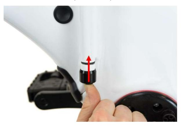
Frame lower hinge bolt retention clip installation - push up firmly as shown
