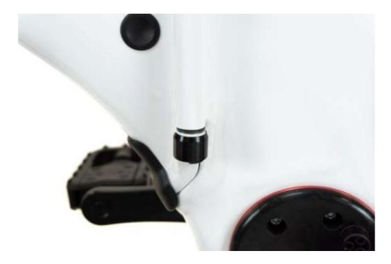
Frame lower hinge bolt retention clip installed - correctly.
