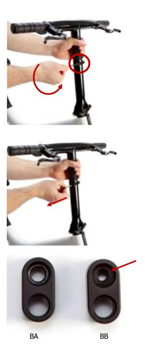
1.1. Depending on the frame number, Use a 4mm Allen key or a Torx T30 to undo the handlebar stem bolt, as shown.
