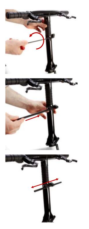
2.1 Unscrew the boltby one completerevolution so both parts,BA and BC, are free tospin.
