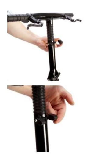
1.6. Locate the threaded hole in Part C (BC) of the pannier rod holder.
