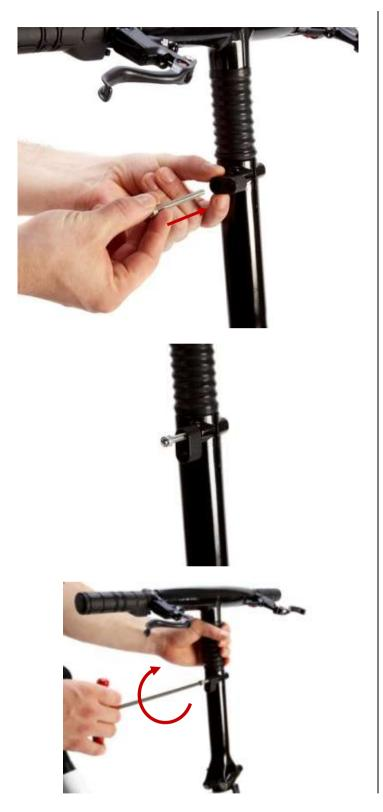
1.3. Insert the M6 bolt (A) into the smaller hole in Part A of the pannier rod holder (BA). Insert the M6 bolt into the Handlebar Stem.
